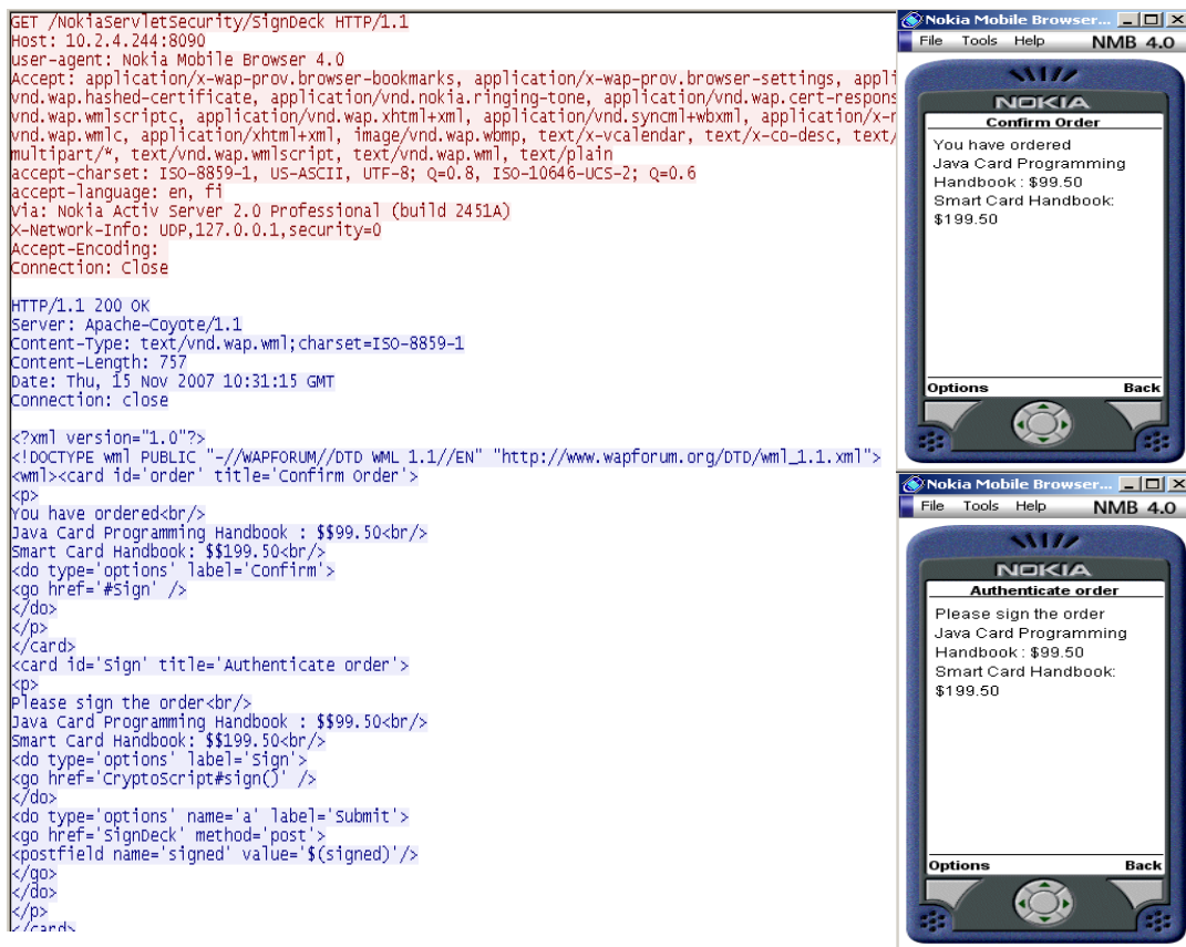
Fig. 7 HTTP Network Analysis for requesting 2 books using a mobile Web WAP application
